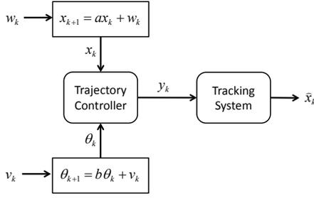
Fig. 1: The trajectory controller and the tracking system at time instant  $k$ .
