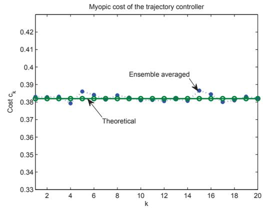
Fig. 2: Myopic cost for the trajectory controller when states evolve in parallel, i.e.,  $a = b$ .
